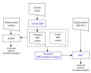
Figure 2. Verification and validation workflow of TASTE models with the BIP framework. Components in blue are new/extended tools developed in the ESROCOS framework.
