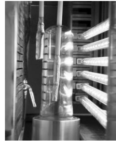
figure 3 : Thermocouples oven' instrumentation (inside the tubular preform and air temperature)
