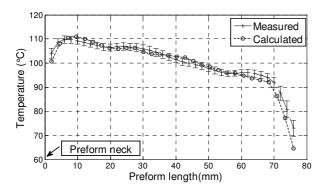
Figure 5: Temperature profile along the preform height
