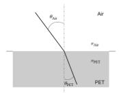
Figure 2: Ray refraction at air-PET interface crossing
