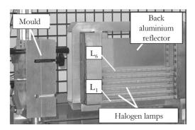
Figure 3: In-lab infrared oven
