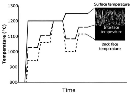
**Figure 3** Thermal gradients across 170  $\mu\text{m}$  thick EB-PVD YSZ and 2 mm thick AM3 substrate.
