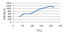
FIGURE 10 Specific heat capacity of the carbon fiber reinforcement
