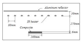
FIGURE 3 Schematic presentation of the IR oven
