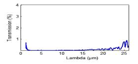
FIGURE 8 Spectral transmission  $T^{\lambda}$  of the carbon reinforcement
