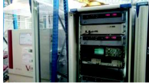
Fig. 2. Test bench: climatic chamber and power electronics
