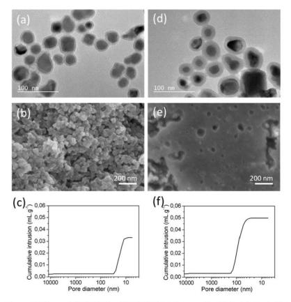
Fig. 2. Transmission Electron Microscopy (TEM) images of a) LSMO@SiO<sub>2</sub>(5) and d) LSMO@SiO<sub>2</sub>(10) starting nanoparticles; High Resolution Scanning Electron Microscopy (HR SEM) of b) LSMO-SiO<sub>2</sub>(5) and e) LSMO-SiO<sub>2</sub>(5) and e) LSMO-SiO<sub>2</sub>(10) composites; Cumulative pore intrusion evolution of c) LSMO-SiO<sub>2</sub>(5) and f) LSMO-SiO<sub>2</sub>(10) composites.
