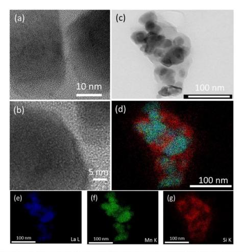
Fig. 3. Characterization of the microstructure of LSMO-SiO<sub>2</sub>(5) composite with a,b) High Resolution Transmission Electron Microscopy (HR TEM) image, c) bright field Scanning Transmission Electron Microscopy (STEM) image, and STEM-EDS (Energy Dispersive Spectroscopy) elemental maps of d) lanthanum, e) manganese, f) silicon. The image g) represents the superposition of La, Mn and Si elemental maps.
