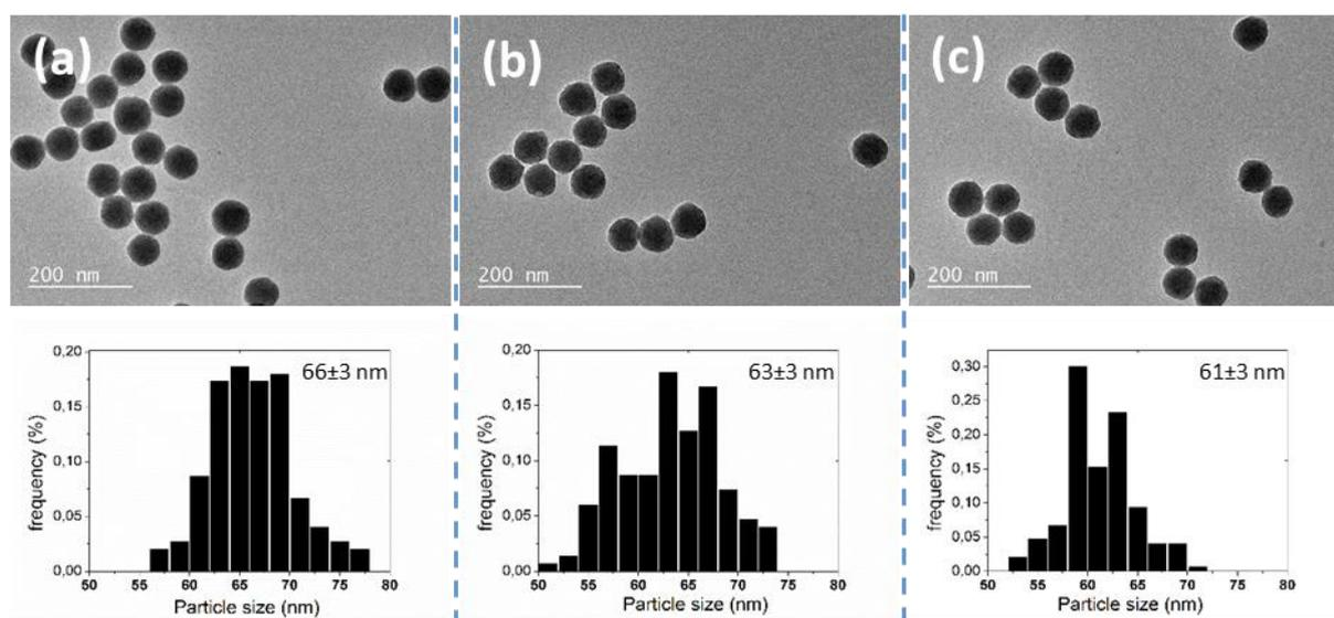
Fig. 2. TEM images of silica nanoparticles and associated statistics on the particle size on a) SiO<sub>2</sub>-NC, b) SiO<sub>2</sub>-200 and c) SiO<sub>2</sub>-400
