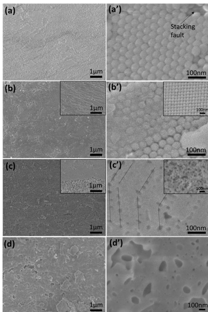
Fig. 7. HRSEM images of (a-a') P-SiO<sub>2</sub>-400, (b-b') P-SiO<sub>2</sub>-200, (c-c') P-SiO<sub>2</sub>-NC and (d-d') P-SiO<sub>2</sub>-AW. For images b' and c', minority microstructures are shown in insert. In figure c', the full lines are just a guide-to-the-eye to emphasize the pore organization.
