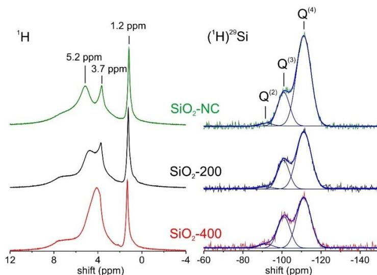
Fig. 5. <sup>1</sup>H MAS and (<sup>1</sup>H)<sup>29</sup>Si CP-MAS NMR spectra of silica nanoparticles
