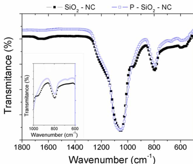
during sintering. The insert focuses on the disappearance of the silanol band at  $953\text{ cm}^{-1}$  and the native Si-O-Si siloxane band at  $670\text{ cm}^{-1}$  in the sintered sample.
