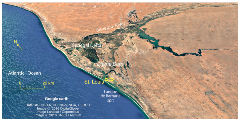
Figure 2. The Senegal River delta, a fine example of a wave-dominated delta characterised by the Langue de Barbarie spit and a river-mouth system subject to strong north-south longshore drift.
