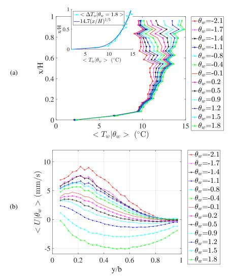
Figure 6: Conditional mean: (a) wall temperature and (b) vertical velocity component averaged over  $0.73 \le x/H \le 0.77$ .
