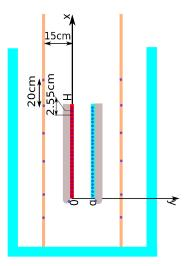
Figure 2: Positions of the thermocouples. The left stainless-steel wall is heated with a constant heat flux. The right polycarbonate wall is adiabatic.
