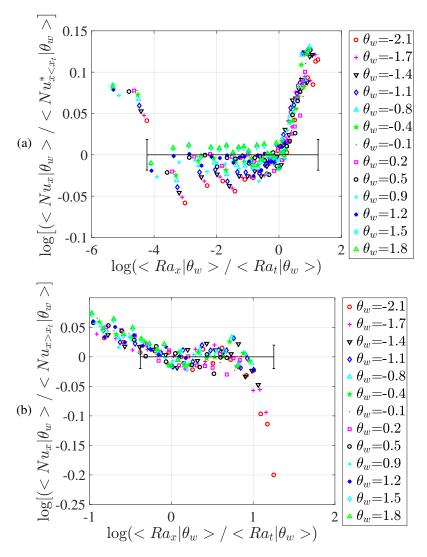
Figure 8: Nusselt–Rayleigh number diagrams conditioned by the value of the average wall temperature. The origin of the horizontal axis corresponds to  $x = \langle x_T | \theta_w \rangle$ . The Nusselt number is compensated by the conditional means of (a)  $Nu_{x < x_T}^*$  (Eq. (10)) and (b)  $Nu_{x > x_T}$  (Eq. (9b))
