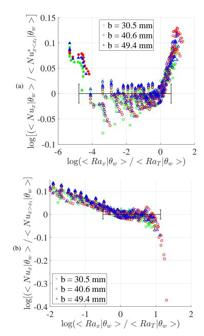
Figure 10: Nusselt–Rayleigh number diagram conditioned by the value of the average wall temperature for the three experiments listed in Table 1. For each value of  $\theta_w$ , the Nusselt number is compensated by (a)  $Nu^*_{x < x_T}$  (Eq. (10)) and (b)  $Nu^*_{x > x_T}$  (Eq. (9b) with  $\alpha = 1.9$ ). Full symbols correspond to the entry of the channel x/H = 0.04. Owing to compensation, the origin of the horizontal axis is  $x = \langle x_T | \theta_w \rangle$ .
