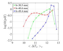
Figure 12: Probability density function (pdf) of the average wall temperature  $\langle \Delta T_w \rangle_x$  for the three channel widths. Only points that correspond to more than 100 measurements are shown.
