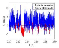
Figure 5: Vertical component of the bulk velocity averaged over  $0.73 \le x/H \le 0.77$  and  $0 \le y/b \le 1$  as a function of time. Red squares correspond to the single-plate mode according to Eq. (3).
