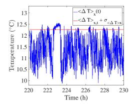
Figure 3: Time evolution of the average wall temperature over a limited timespan corresponding to the velocity measurement time. The horizontal line represents  $\langle \Delta T_w \rangle_{x,t} + \sigma_{\langle \Delta T_w \rangle_x}$ .
