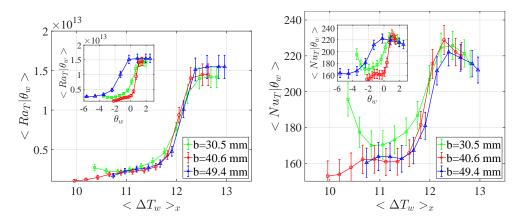
Figure 11: Conditional means of the Rayleigh number (a) and the Nusselt number (b) at the transition point as functions of the mean wall temperature. The insets show the same quantities as functions of the reduced wall temperature.
