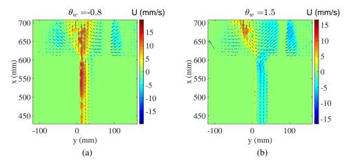
Figure 7: Conditional mean of the velocity field for (a)  $\theta_w = -0.8$  and (b)  $\theta_w = 1.5$ . The background color represents the vertical component U. The heated plate is on the left.
