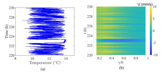
Figure 4: (a) Evolution of the wall temperature at x/H = 0.75 for the time period t = 220.1-230.1 h during which velocities are measured. (b) Temporal evolution of the instantaneous vertical velocity profile averaged over  $0.73 \le x/H \le 0.77$  for t = 220.1-230.1h.
