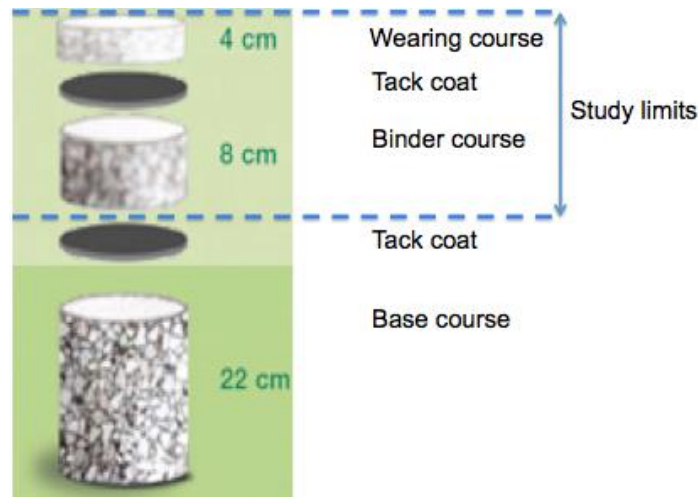
Figure 1: Tack coat positioning in a pavement structure.
