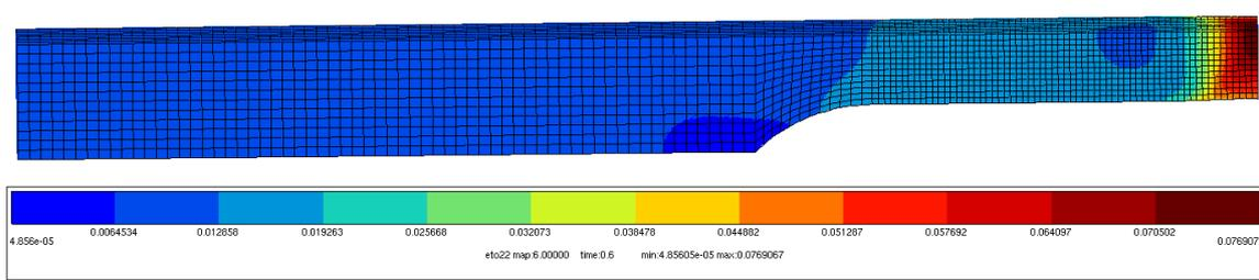
Figure 6: Similar *Ti17-Ti17* LFW joint tensile test simulation.
