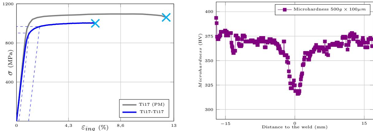
Figure 3: Tensile test curves comparison of the *Ti17* parent material and the *Ti17 - Ti17* similar welding. Parent material information has been provided by [Millet and Wies. (2015)]. Microhardness line perpendicular to the weld line.
