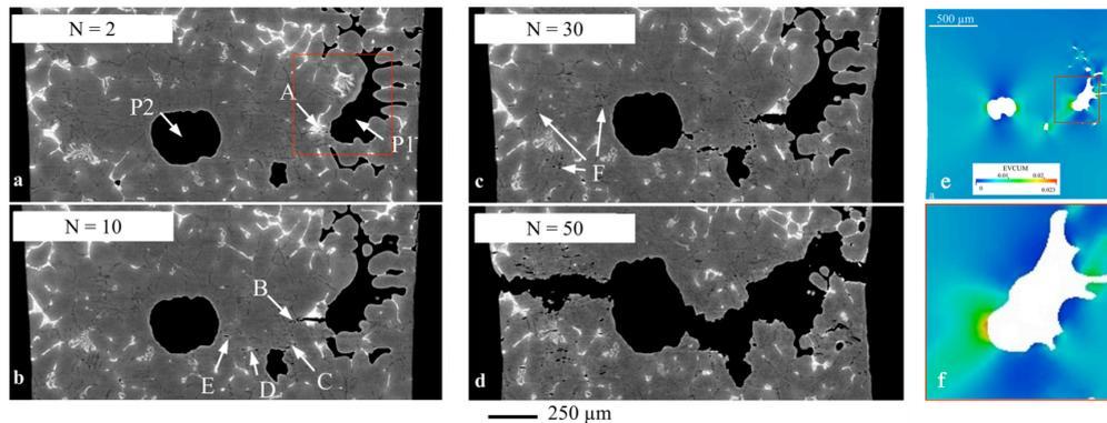
**Figure 2.** (a) to (d) Tomographic slices showing the evolution of the damage for Lost Foam Casting Aluminium alloy. The labels on subfigures show pores (P1 and P2) or broken particles (A to E) ; (e) cumulated inelastic strain, mesh corresponds to (a) and (f) detailed view [12]
