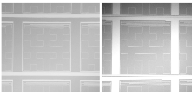
Fig. 3. Left: a front-illuminated microstrip (MS) pixel for the 260 GHz band of NIKA2. The pixel size is 2 \times 2 \text{ mm}^2 . Right: a back-illuminated coplanar waveguide (CPW) pixel used for the 150 GHz band in NIKA. The pixel size was in that case 2.3 \times 2.3 \text{ mm}^2 . Both designs are based on Hilbert-shape absorbers/inductors.
