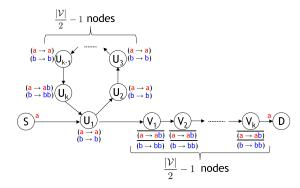
Fig. 2. Example of multi-layer network in which the only feasible path is of length  $\Omega(n^2)$ .
