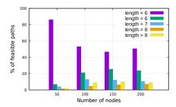
Fig. 7. Feasible path length distribution with p = 0.05.
