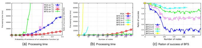
Fig. 8. Processing time of PDA and BFS on scale free topologies and ratio of success of BFS according to the network size.
