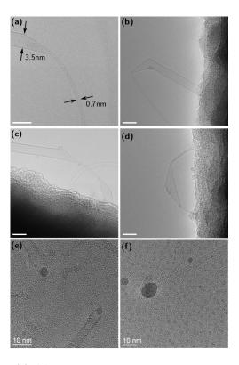
FIG. 3. (a)-(d) TEM images of SWNT intramolecular junctions formed by alternating CO and  $\mathrm{CH_4}$  during CVD growth processes at 1073 K. Scale bars in all images are 5 nm. TEM images of SWNTs grown by (e) tangential mode by  $\mathrm{CH_4}$  and (f) perpendicular mode by CO at 1073 K.
