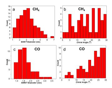
FIG. 1. (Color online) (a) Diameter and (b) chiral angle distributions of SWNTs grown on Fe nanoparticles at 1073 K using CH<sub>4</sub> as the carbon source. (c) Diameter and (d) chiral angle distributions of SWNTs grown on Fe nanoparticles at 1073 K using CO as the carbon source.
