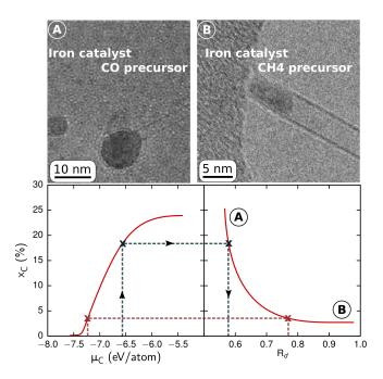
FIG. 5. (Color online) Top: TEM images of tubes grown by perpendicular (A) or tangential (B) growth modes. Bottom: Sketch of the relation between the chemical potential of carbon atoms delivered at the surface of the NP ( $\mu_c$ ), controlled by the precursor decomposition reaction, and the growth mode  $R_d$ , via the carbon fraction  $x_c$  in the NP. The left curve is a carbon sorption isotherm, as calculated in Diarra et al.[37].
