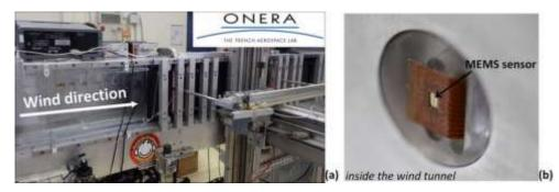
Figure 9: Turbulent boundary layer wind tunnel in ONERA Lille (b) Flush-mounted IEMN MEMS sensor in the wind tunnel wall
