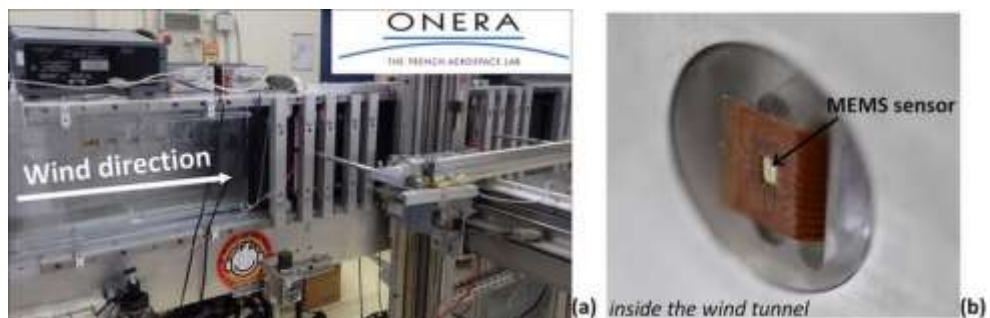
Figure 9: Turbulent boundary layer wind tunnel in ONERA Lille (b) Flush-mounted IEMN MEMS sensor in the wind tunnel wall
