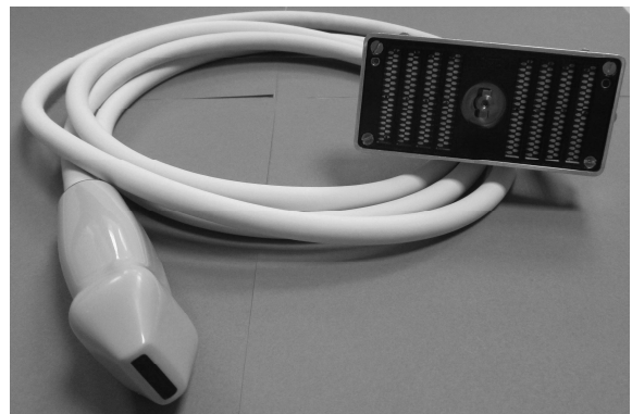
Fig. 3 : Photograph of the complete 128 elements array
