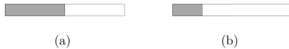
Figure 17: In 1D composite materials can either be (a) centro-symmetric (isotropic) or (b) non-centro-symmetric (hemitropic).
