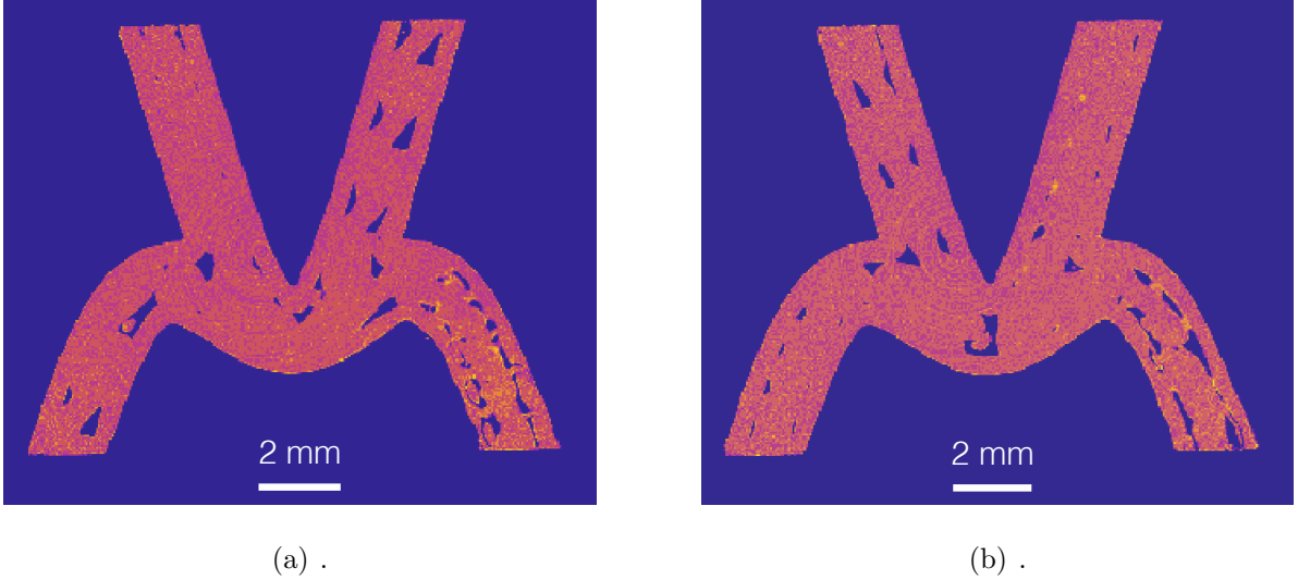
Figure 11: Tomographic images of a [Z_2^\pi] cell obtained by FDM, corresponding to two successive slices of the process. The 1048 \times 1223 \times 1121 voxels images are obtained with the LMT X-ray lab-CT.
