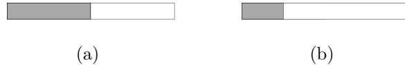
Figure B1: In 1D composite materials can either be (a) centro-symmetric unit cell (isotropic) or (b) non-centro-symmetric unite cell (hemitropic).
