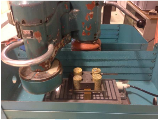
a) Mechanical surfacing
