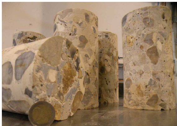
Fig. 20. Concrete samples of 103 mm diameter
