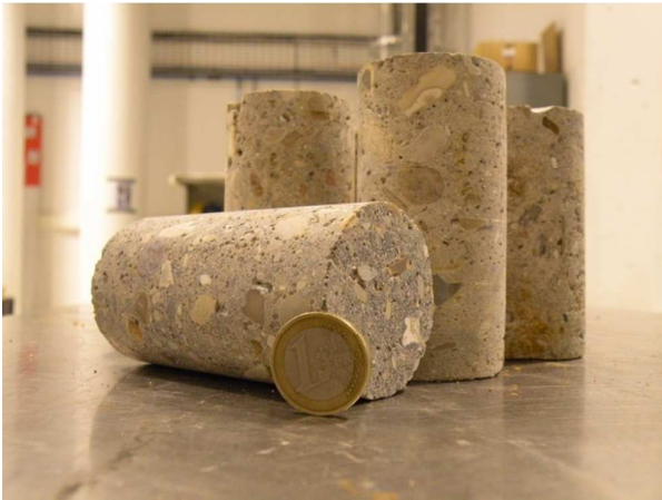
Fig. 9. Mortar samples of 50 mm diameter
