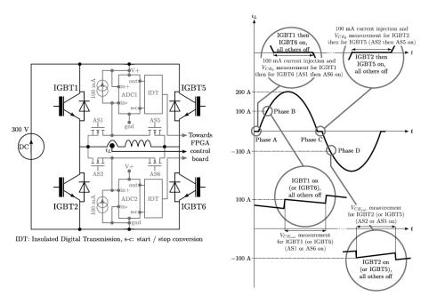
Fig. 8 [22]: Implementation strategy for Voltage at Low Current in a single phase inverter: Temperature measurement is taken when load current crosses 0A
