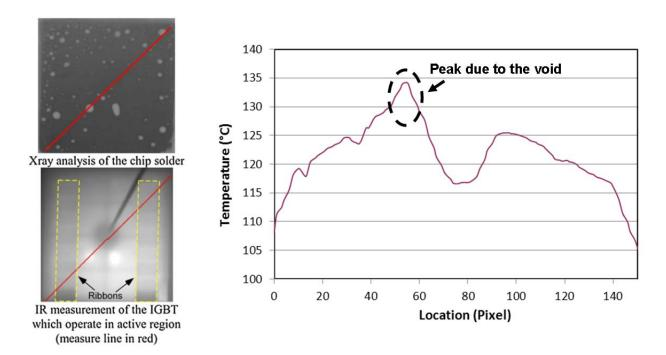
Fig. 7: Temperature distribution in an IGBT chip with peak temperature caused by a solder void
