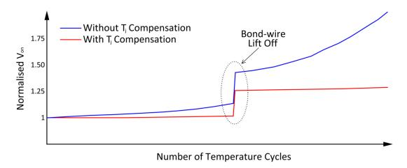
Fig. 3: Evolution of  $V_{on}$  with and without temperature compensation
