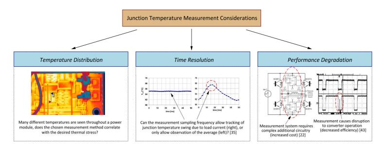
Fig. 6: Considerations for selection and design of a junction temperature measurement system
