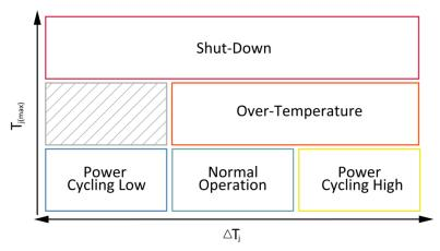
Fig. 5 [28]: Control strategies defining different thermal operating regions based on junction temperature swing  $(\Delta T_j)$  and maximum junction temperature  $(T_{j(max)})$
