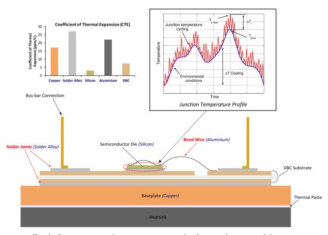
Fig. 1: Cross-section and construction materials of a typical power module
