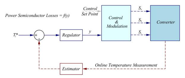
Fig. 4: Example of active thermal control of power semiconductor junction temperature,  $T_j$ , by means of y (switching frequency, reactive power or any other quantity that can modify the power semiconductor losses).  $T_j$  is obtained using an estimator based on an online temperature measurement method.
