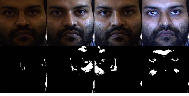
Fig. 3. Specular highlight detection results on images under various lighting conditions. Top: raw images; bottom: detected highlight masks.
