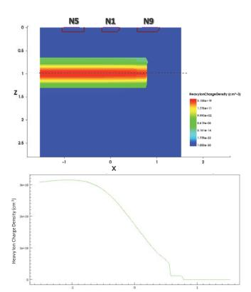
Fig. 7. 2D heavy ion charge density and 1D variation of the heavy ion charge density.
