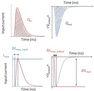
Fig. 3. Definition of the characteristics of the input and output signal.
