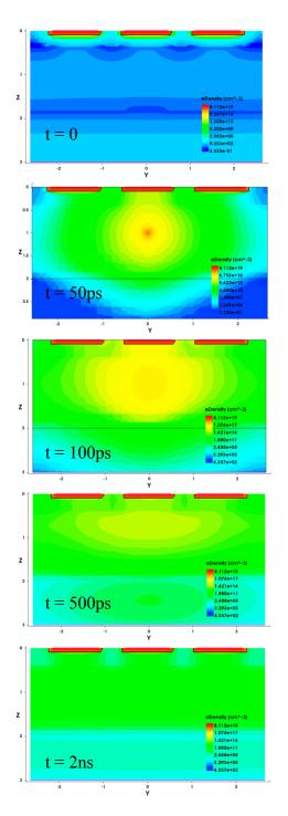
Fig. 8. Evolution of electron density in the Y direction.
