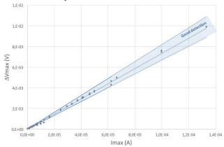
Fig. 4. Variation of the average output signal ( $\Delta V_{max}$ ) versus the maximum of the input current ( $I_{max}$ ).
