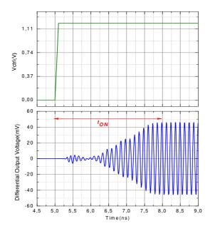
Fig. 9 Post layout simulated LNA differential output voltage.
