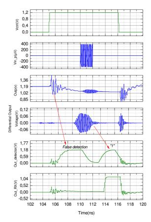
Fig. 10 Post layout simulated receiver waveforms.
