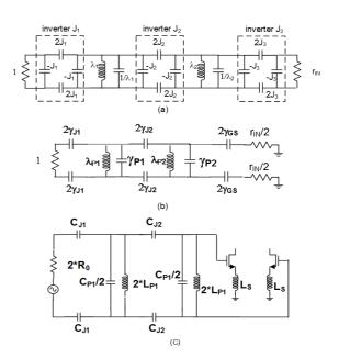
Fig. 4 Fully differential input matching cell: (a) Normalized (by  $R_0=50\Omega$  and  $\omega_0$ ) differential LC ladder filter with capacitive admittance inverters, (b) Normalized input matching cell. (c) Input matching cell implementation.
