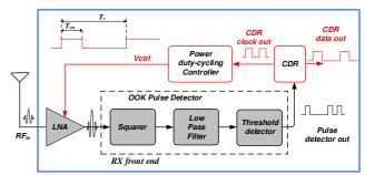
Fig. 1 Self synchronized and duty-cycled receiver architecture.
