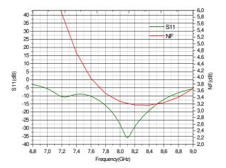
Fig. 8 The return loss S11 and the noise figure.
