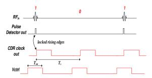
Fig. 2 Input and output receiver signals in the steady state duty-cycled mode.
