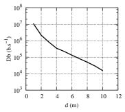
Figure 8. Mean bit rate as a function of the communication range.
