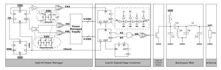
Figure 5. Pulse generator design
