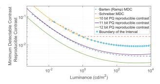
Fig. 2. Minimum detectable contrast thresholds and reproducible contrast curves of 10-bit, 11-bit and 12-bit PQ.
