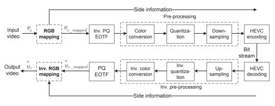
Fig. 1. Diagram of the recommended HDR video coding system with proposed modifications.
