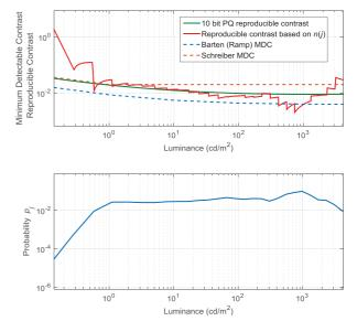
Fig. 4. The probability p(j) and the reproducible contrast based on n(j) with 10-bit depth codewords.
