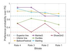
Fig. 15. Preference probability of selecting the proposed version over PQ, when HM 16.2 is used. Rate 4 < Rate 3 < Rate 2 < Rate 1.
