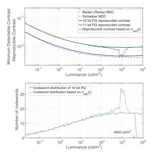
Fig. 5. Reproducible contrast and codeword distribution based on  $n_{adp}(j)$  with 10-bit depth.
