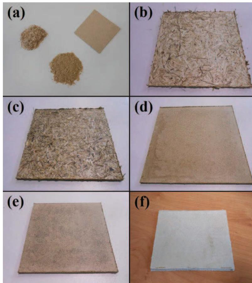
**Figure 1.** Photographs of (a) starting materials used for thermo-pressing (i.e., raw shives, extruded shives and handsheet obtained from extruded shives, from left to right), (b) RS board, (c) RSL board, (d) ES board, (e) ESL board, and (f) HS board.
