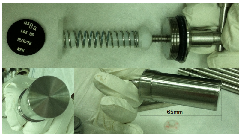
Figure 5. The source holder that connects to an arm and to the articulation gear of the deployment device. The source, here a ^{133}\text{Ba} source, is pressed to the tip of the source holder via a spring.
