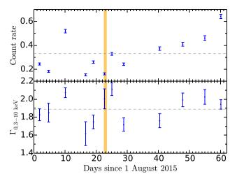
**Figure 4.** Upper panel: *Swift* XRT 0.3–10.0 keV count rates in counts s<sup>-1</sup>. Lower panel: The X-ray photon index  $\Gamma$  of the best-fitting absorbed power-law model fit to the *Swift* spectrum. The mean values of both count rate and  $\Gamma$  are shown as grey dashed lines. The time span of the *XMM–Newton* observation is highlighted in orange.
