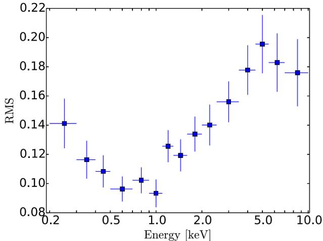
**Figure 3.** The X-ray RMS fractional variability spectrum of 1H 0323+342. Fifteen light curves spanning the 0.2–10.0 keV energy range were created from the *XMM–Newton* EPIC pn event file with time bins of 500 s.
