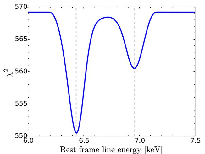
**Figure 6.** Variation in the  $\chi^2$  fit statistic with the rest frame line energy of a narrow (fixed width  $\sigma = 10$  eV) Gaussian emission line. Best-fitting line energies of 6.43 and 6.95 keV are indicated with dashed lines.
