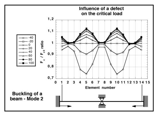
Figure 5: Influence of a defect on the critical load
