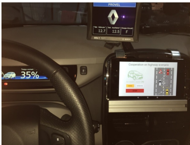
Figure 6: Human Machine Interface implemented on an Android based tablet.
