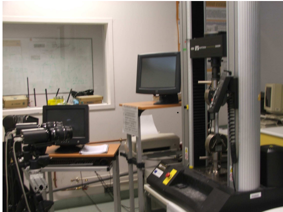
FIGURE 1. DISC set up and tensile testing machine
