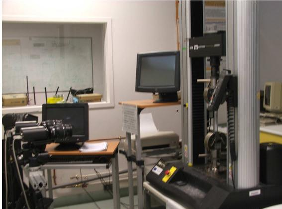
**FIGURE 1.** DISC set up and tensile testing machine
