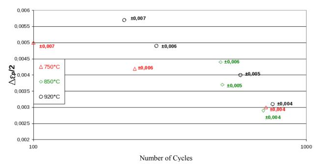
Fig. 7: Lifetime fatigue results performed on GX30NiCr39-24 steel
