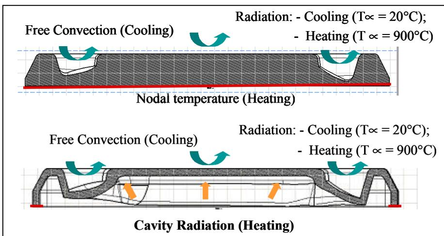
Fig. 12 : Numerical simulation applied to die optimization
