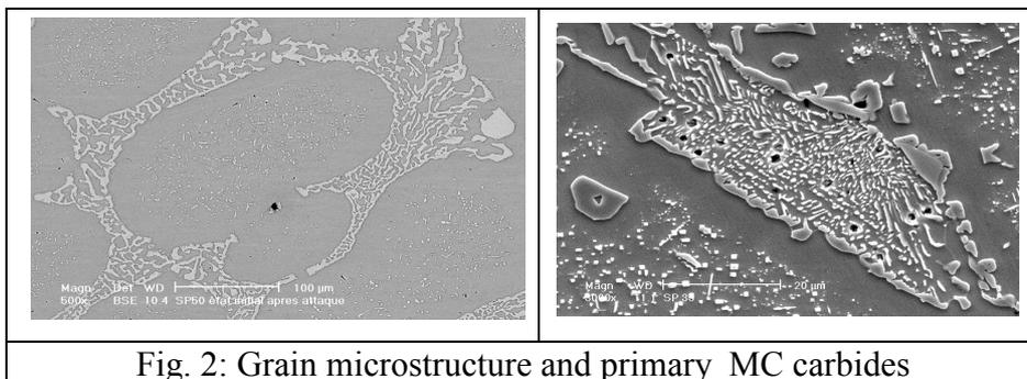
Fig. 2: Grain microstructure and primary MC carbides
