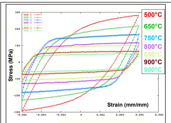
Fig. 6: Stress-strain fatigue loops for increasing temperature ( $\dot{\epsilon} = 10^{-3} s^{-1}$ )
