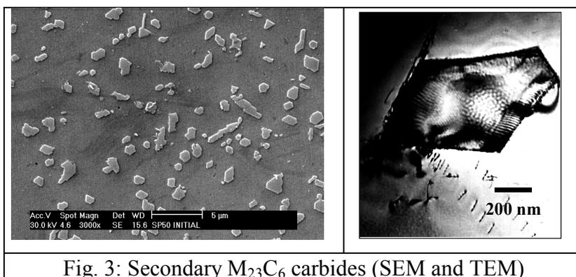
Fig. 3: Secondary  $M_{23}C_6$  carbides (SEM and TEM)
