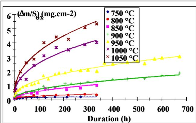
Fig. 9 : Oxidation kinetics of 50% Ni HR Steel
