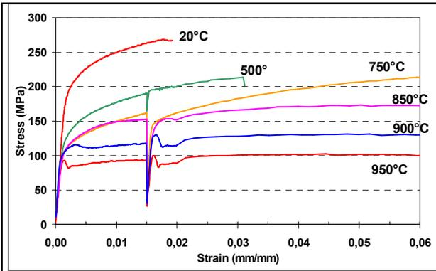
Fig. 4: Tensile testing with relaxation (columnar zone,  $\dot{\epsilon} = 10^{-3} s^{-1}$ , 50% Nickel)
