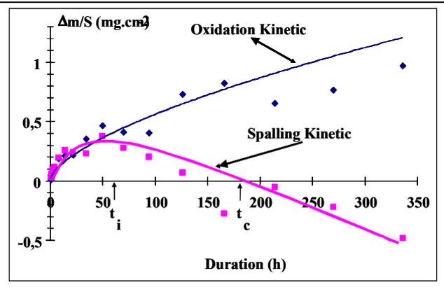
Fig. 10 : Spallation kinetic of 50% HR Steel
