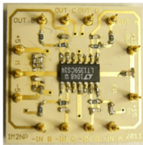
Figure 2 Home built in situ transimpedance preamplifier, current-voltage conversion by 2.2 k \Omega resistances, bandwidth 5 MHz. The chip is a LT1359 (Linear technology) four-operationnal amplifiers circuit.
