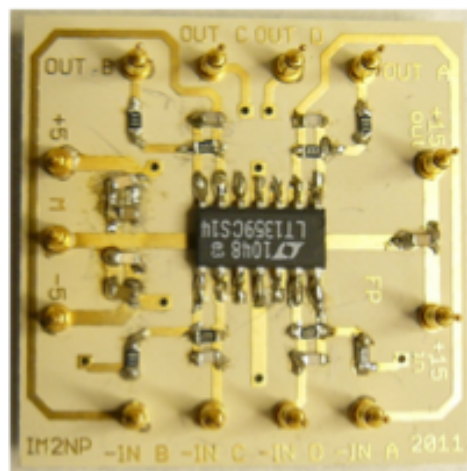
Figure 2 Home built in situ transimpedance preamplifier, current-voltage conversion by 2.2 k \Omega resistances, bandwidth 5 MHz. The chip is a LT1359 (Linear technology) four-operational amplifiers circuit.
