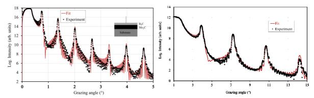
**Figure 2.** Grazing incidence x-ray reflectivity at 8000 eV (left) and at 1500 eV (right): experimental measurements (dots) and numerical adjustment (continuous) with a model of two layers in the period The expected thickness of  $B_4C$  and  $Mo_2C$  was respectively 5 and 2.5nm. The figure in the inset presents the model of two layers in the period:  $B_4C/Mo_2C$ .
