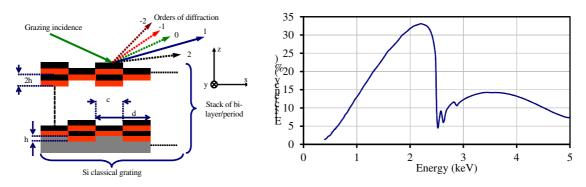
**Figure 1.** A transversal cross section of AML grating which is constituted of  $B_4C/Mo$  multilayer deposited on a laminar grating (figure at left). An example of simulation using the following grating features: 2400 lines/mm, etched depth h=2.5 nm, periods along z axis =30, cyclic ratio c/d= 0.5 (where c is the valley width).
