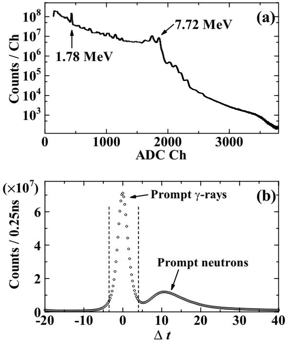
Figure 2. (a) A  $\gamma$ -ray spectrum taken by the  $\text{LaBr}_3(\text{Ce})$  scintillator. The spectrum was obtained without imposing any gate conditions. (b) Time difference ( $\Delta t$ ) between the FFs and  $\gamma$ -rays. Dashed lines indicate the example of gate position (for  $\text{ADC ch} \leq 1000$  ch), which was used to obtain the  $\gamma$ -ray spectrum coincidence with FFs shown below.
