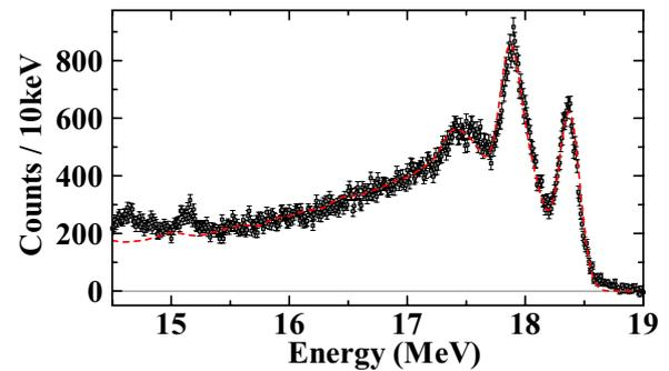
**Figure 4.** Measured 18.4 MeV  $\gamma$ -ray spectrum of the  $^{11}\text{B}(p, \gamma)^{12}\text{C}$  reaction (black square) compared to the calculated one (dotted line) by GEANT4. The calculated spectrum deviates from the measured one below about 15.3 MeV due to the 15.1 MeV  $\gamma$  ray from the same reaction.
