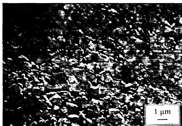
Fig. 4. SEM image of the wear track formed on the diamond coating of Fig. 1 after a tribological test performed at several applied loads (1, 3, 13 N) and  $0.02 \text{ m s}^{-1}$ .
