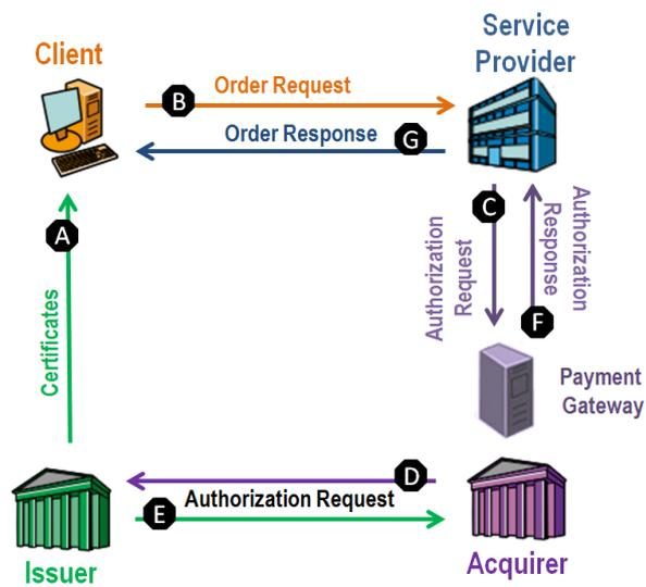
**Fig. 2** The SET protocol (adapted from [31])
