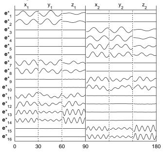
Figure 10. Rotated eigenvectors  $\mathbf{e}_k^*$  associated with the 16 largest eigenvalues  $\lambda_k^*$  in Fig. 9.
