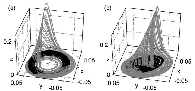
Figure 4. Reconstruction of the leading pair, i. e. RCs 1-2 (black curve), of the coupled Rössler oscillators' actual trajectory (gray curve) in (a) a phase-coherent regime with  $\alpha = 0.15$ ; and (b) in the funnel regime with  $\alpha = 0.28$ .
