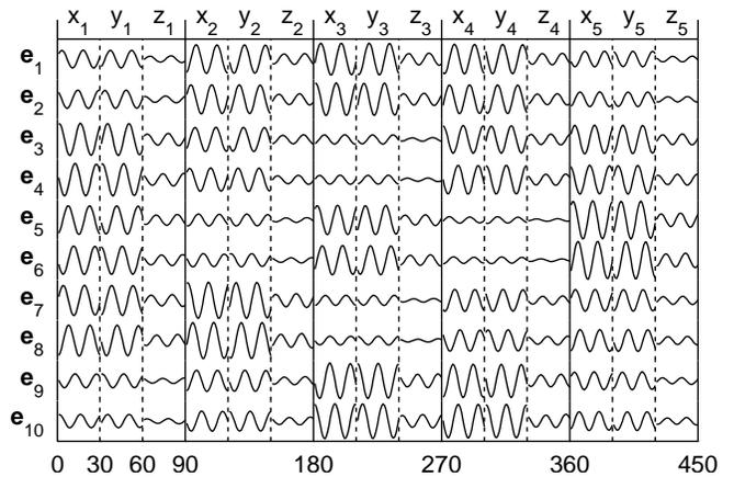
Figure 2. Eigenvectors  $\mathbf{e}_k$  corresponding to the 10 largest eigenvalues  $\lambda_k$  in Fig. 1. Each eigenvector of length  $DM$  is composed of  $D = 15$  consecutive segments, each of length  $M = 30$ , associated with the 15 channels.
