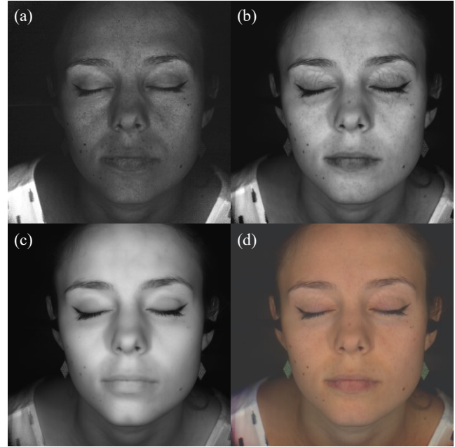
Figure 12. Example of hyperspectral image: (a) Image at 420 nm, (b) image at 590 nm, (c) image at 700 nm, (d) RGB color reconstruction under a D65 illuminant.
