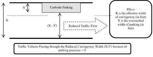
FIG. 3. TRAFFIC FLOW IN PRESENCE OF CURBSIDE PARKING
