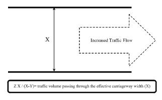
FIG. 4. TRAFFIC FLOW IN ABSENCE OF CURBSIDE PARKING
