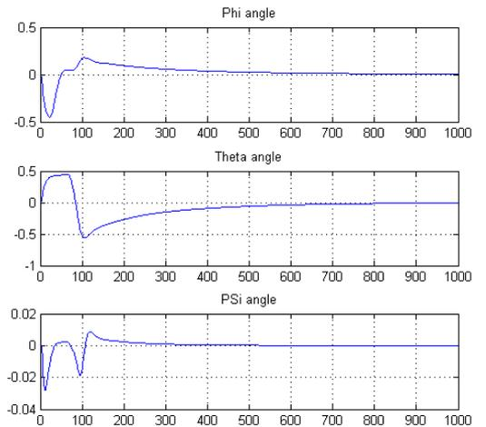
Figure 5: Attitude regulation signals of Quadrotor.
