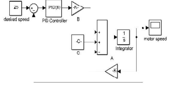
Figure 2: Simulink model of DC-motor
