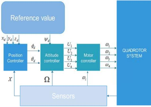
Figure 3: Block diagram of the used control structure
